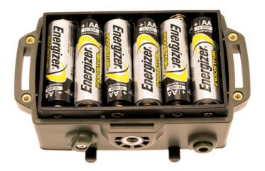
Use a screwdriver to remove the four screws on the back of the device and take off the back wall. Insert six AA batteries into the battery holder, taking care to follow the polarity direction indicated on the holder. Check the sensor turns on and then replace the back wall and the four screws. When replacing the back wall, ensure that the seal around the edge is clean and free of debris.
