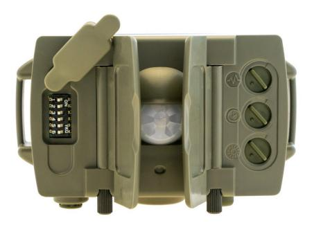
The PIR is configured via three dials and a bank of six switches on the front. There is also an On-off switch on the bottom of the device.
