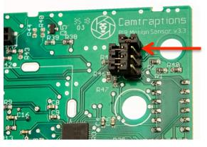
Left: Jumpers A to D in the Off position with jumper connectors stowed on just the right pin.
