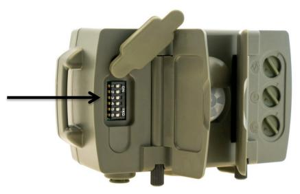
Programs are set via Switches 1 to 6 on the front of the device. These switches are located under the watertight bung, behind the flap, to the left of the sensor dome.
