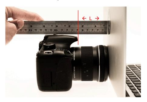
Pick a lens tube based on your length measurement ("L"):
