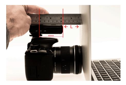
If you don't have a wireless transmitter yet, measure to the front of the hot shoe instead and then subtract 60mm:
