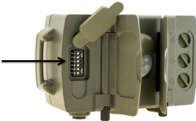
Programs are set via Switches 1 to 6 on the front of the device. These switches are located under the watertight bung, behind the flap, to the left of the sensor dome.
